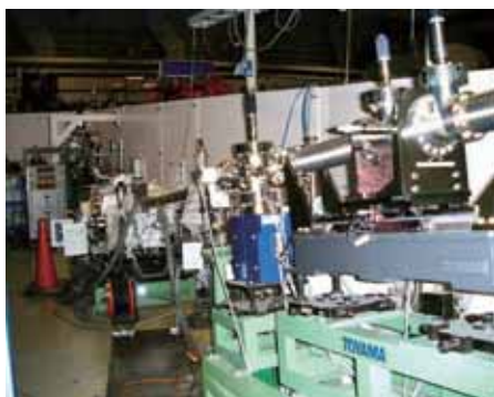
Fig. 1. 18-m spherical grating monochromator at BL2B.
